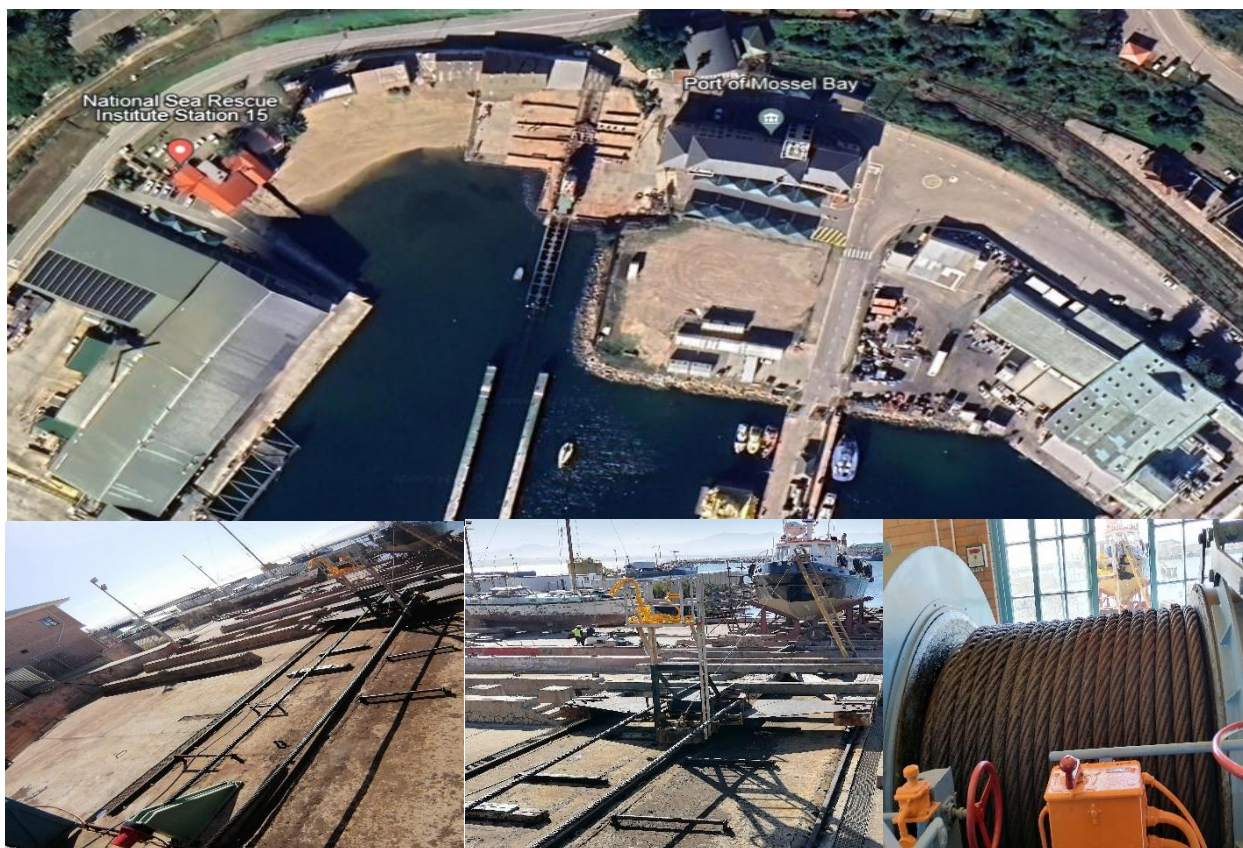
Figure 1: Aerial photo of a slipway facility and the cable on the drum and route around the sheave to the load cell.
